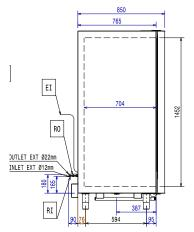
Drain Electrical inlet (power) RO Refrigerant Outlet
